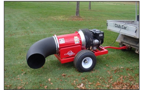
A power blower, used by Middle Smithfield Township's Public Works Department for Dirt and Gravel Road Maintenance
