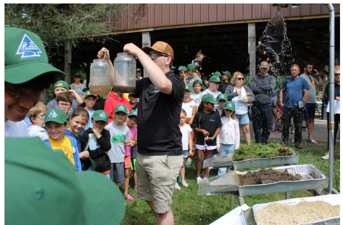
MCCD's Watershed Specialist, Charles Kelshaw, using a rain simulator to demonstrate the differences in runoff and soil infiltration of various land use types
